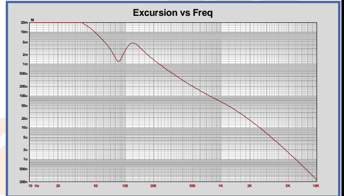
Cone Displacement at 1000W
